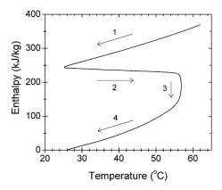
Fig. 7. Enthalpy-temperature diagram for supercooling sodium acetate reconstructed from the temperature plot in Fig. 6. The arrows indicate time in the experiment: (1) initial cooling of liquid phase, (2) crystallization, (3) release of latent heat, and (4) finally cooling of the solid phase to room temperature.
