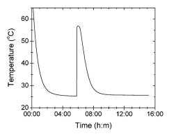
Fig. 6. Temperature as a function of time as the sodium acetate becomes supercooled, crystallizes, and cools again.
